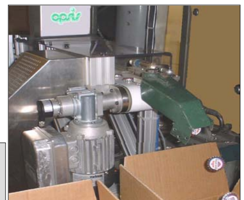
Crown cork testing on the conveyor
